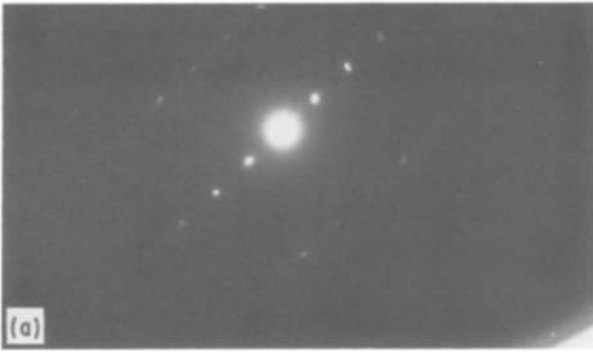
Figure 4 (a) Transmission electron micrograph of unfaulted region of x-phthalocyanine crystal with the associated diffraction pattern. (b) Tracing of the diffraction pattern of 4(a).
